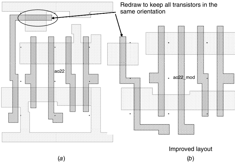
Figure 10.5 (a) Layout with transistors drawn both vertically and horizontally. (b) Improved layout.
